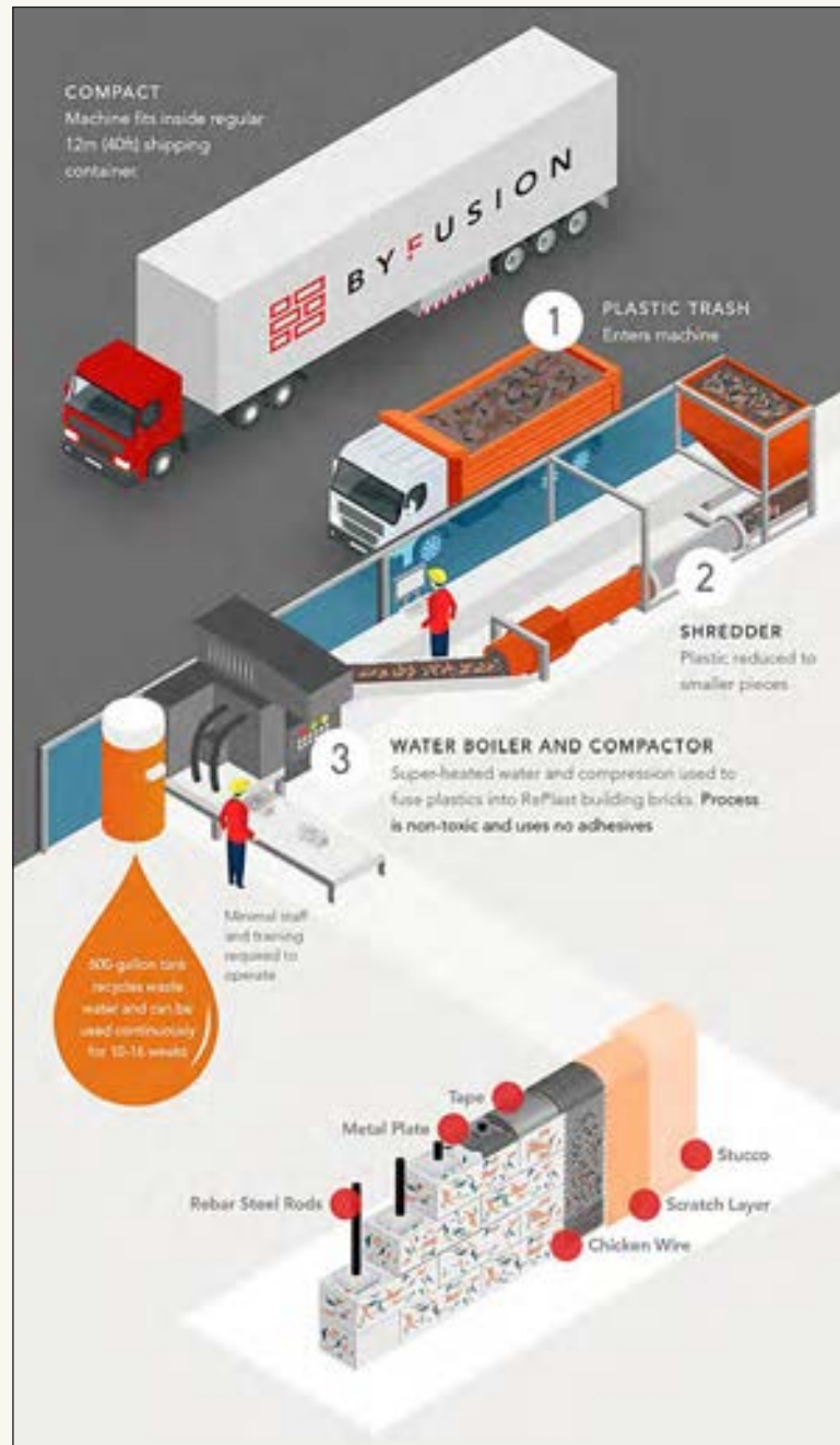
FIGURE 8. BYFUSION'S PROCESS TO MAKE BUILDING BLOCKS FROM PLASTIC BOTTLES
