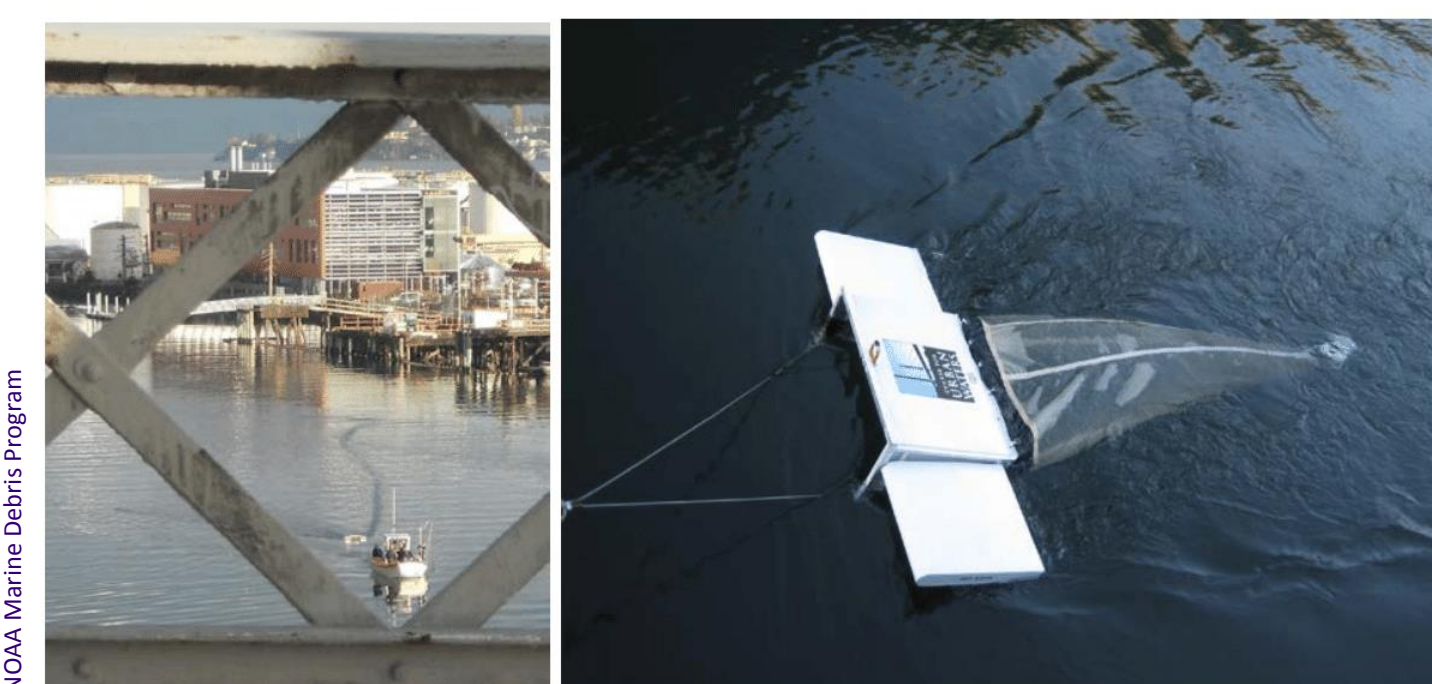
Figure 1. Researchers use a manta net to collect surface water samples in the Thea Foss Waterway, Puget Sound, Washington.
