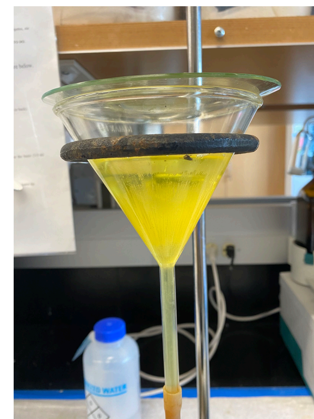
FIG 5. Density Separation II. Buoyant microplastics prepared for collection
