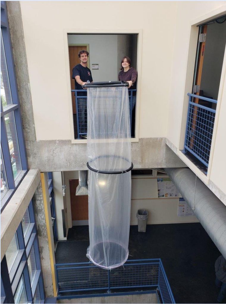
Figure 3: The mesocosms were pre-built in the lab and placed in Lake Killarney, WA, with different concentrations of lanthanum-modified bentonite (EutroSORB G).
