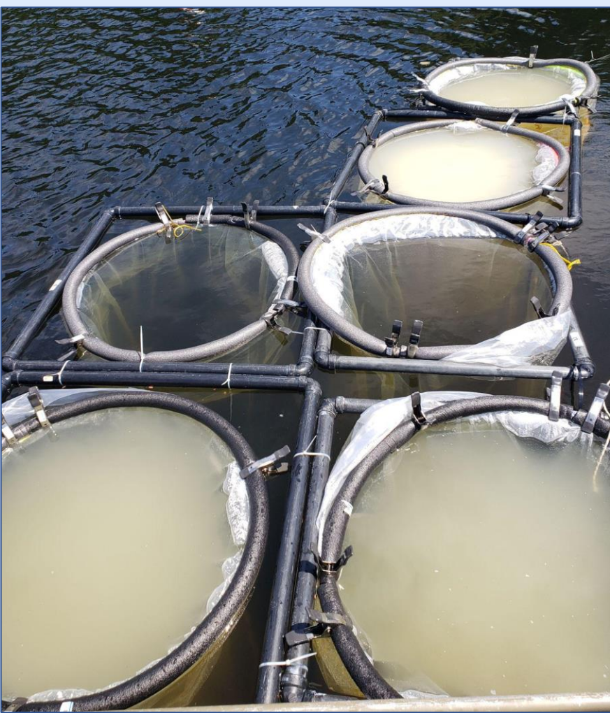
Figure 3: The mesocosms were pre-built in the lab and placed in Lake Killarney, WA, with different concentrations of lanthanum-modified bentonite (EutroSORB G).
