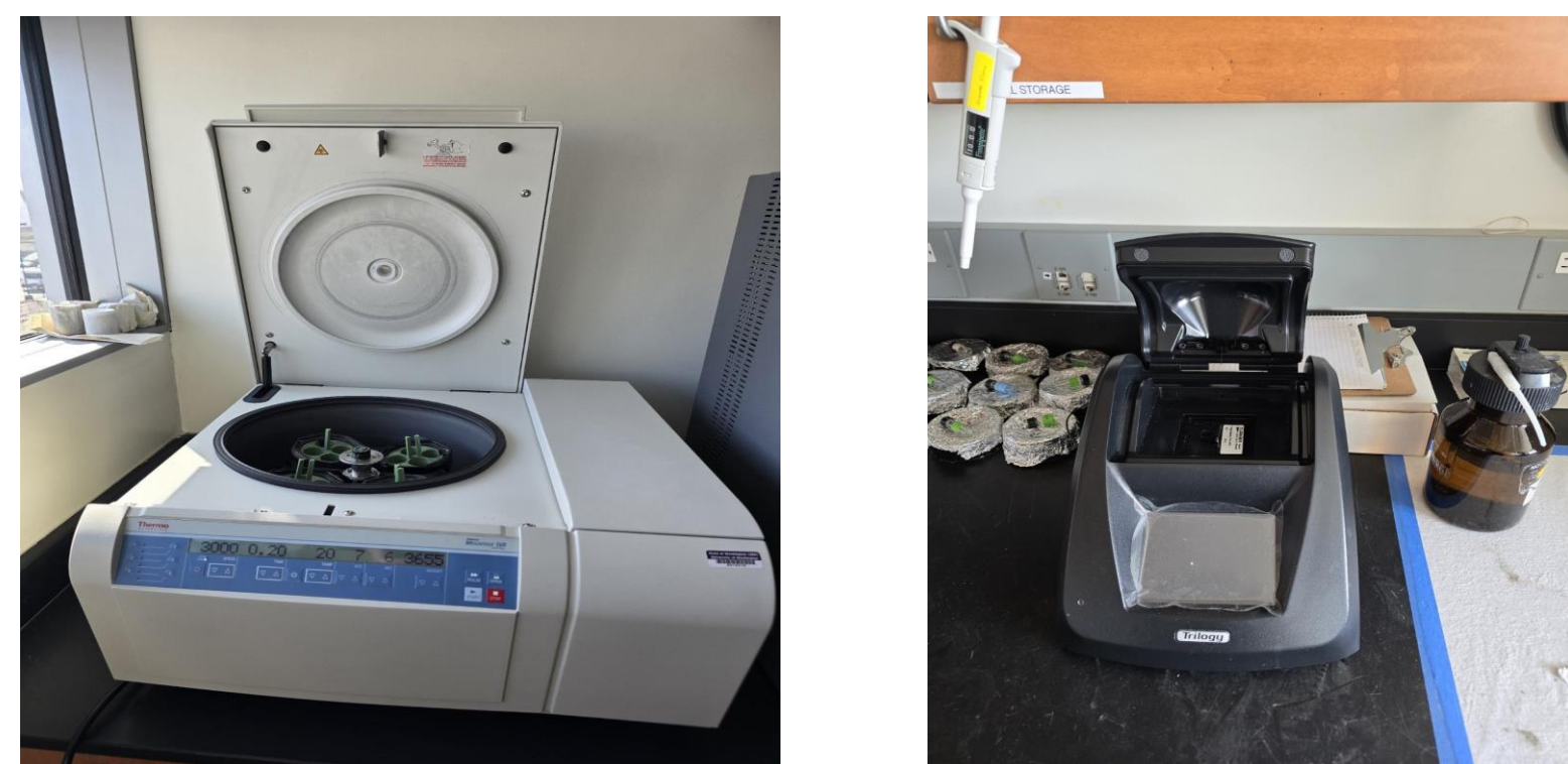
Figure 1: Images of Centrifuge and Fluorometer used for separation and fluoresent analysis of chlorophyll-a concentration.
