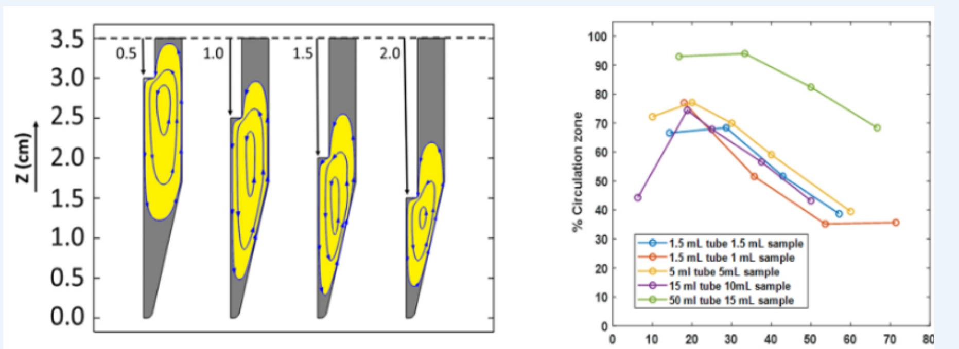
**Modeling effect of tip depth on mixing.** ( Ferdous et. al 2021). The yellow area indicates circulation zone. The line graph illustrates the percentage of volume in circulation zone with changing tip height for four sizes. This figure is from a sonication optimization study that led us to alter our protocol to try and increase lysis efficacy based on their results. (2)
