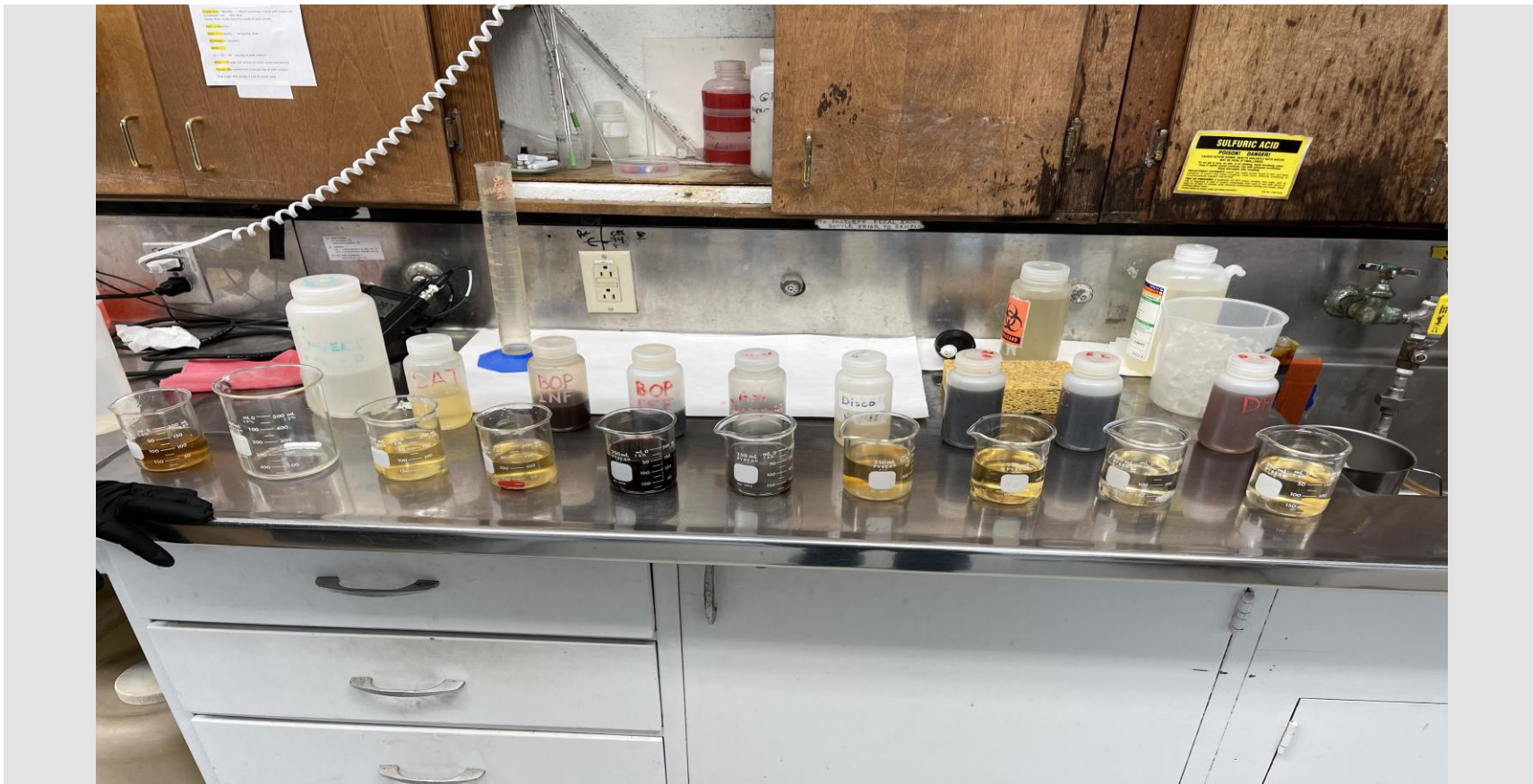
Image 1: Water samples from various waste streams in the plant. Several tests are run on these including a five-day Biological Oxygen Demand test.
