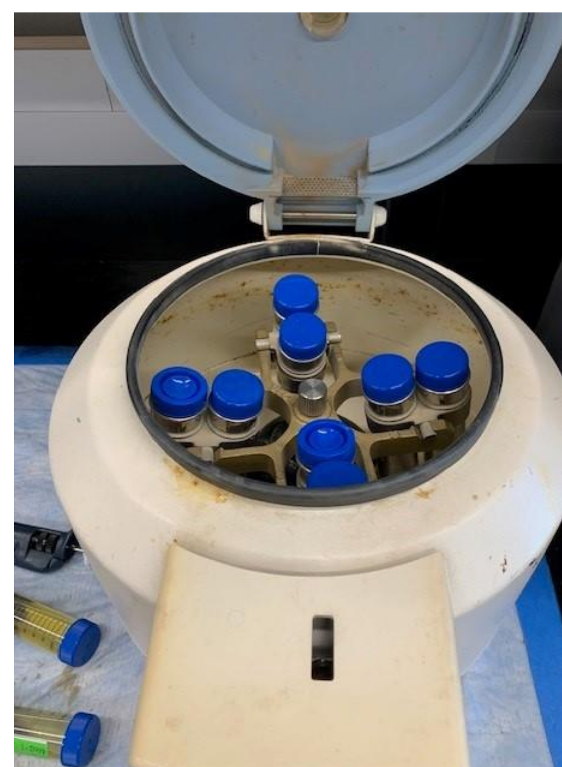
Figure 3: Centrifugation after thawed (25 minutes at 3000 RPM), to then be processed with the fluorometer (Photo credits to Eva Marino)
