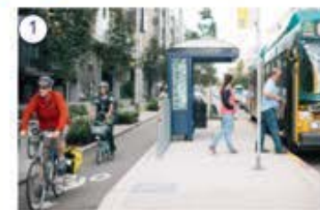
1 Bus Stop Seattle, WA - Accessible design - Floating bus island - Limited vehicle access
